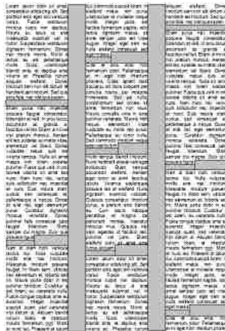
Figure 2.23: White-space analysis finds set of rectangles that comprise white space within the document. The gray rectangles indicate white space.
