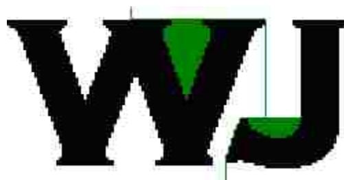
Figure 2.17: The execution of the path-finding algorithm to find the white space between characters.
